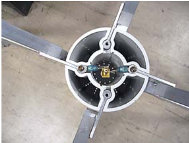
Figure 4. New antenna with short 1/8" diameter leads to measurement point.
