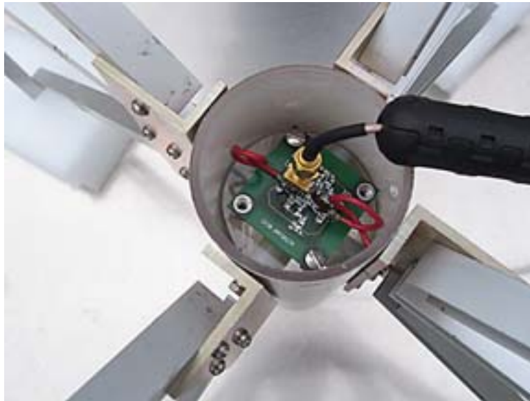
Figure 2. Original MWA Antenna with single turn coil plus connection pads on original pc board.
