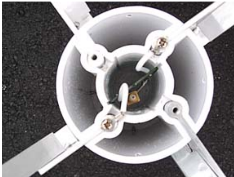
Figure 5. New antenna including the new pc board. The impedance was measured at pads at the ends of the traces to the transistor inputs.
