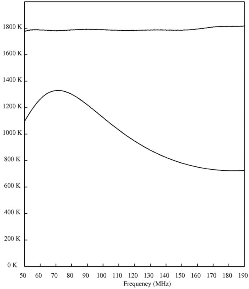
Figure 3. Upper and lower curves are the calibrated and uncalibrated spectra of the “hot filament” source respectively.
