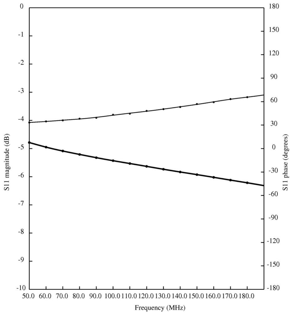
Figure 2. Reflection coefficient of “hot filament” source. Lower curve is the phase.
