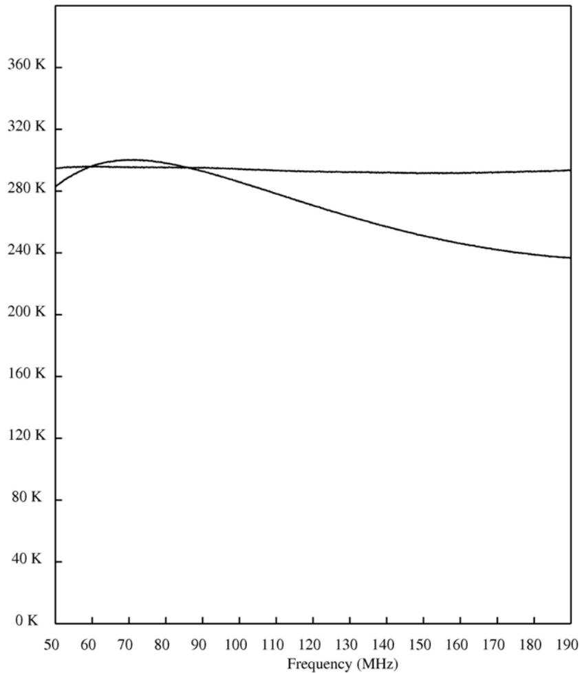
Figure 1. Upper and lower curves are the calibrated and uncalibrated spectra of the 6 dB “open ended” attenuator.
