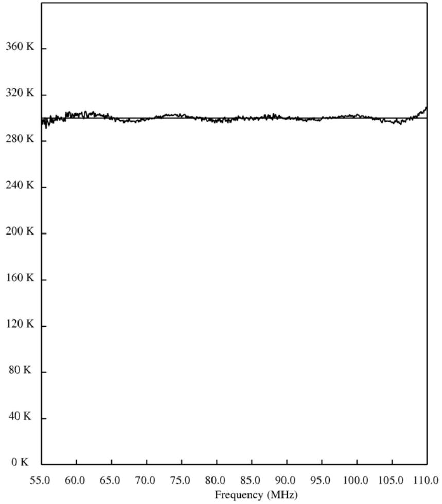
Figure 4. Upper and lower curves are the calibrated and uncalibrated spectra from the open cable.
