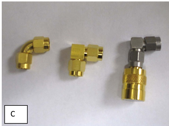
Figure 5. A extension to shield open end, B: Balun with bends attached to VNA and shorted, C: SMA bends tested, D: Balun terminated with 47\Omega resistor, E: Balun shorted
