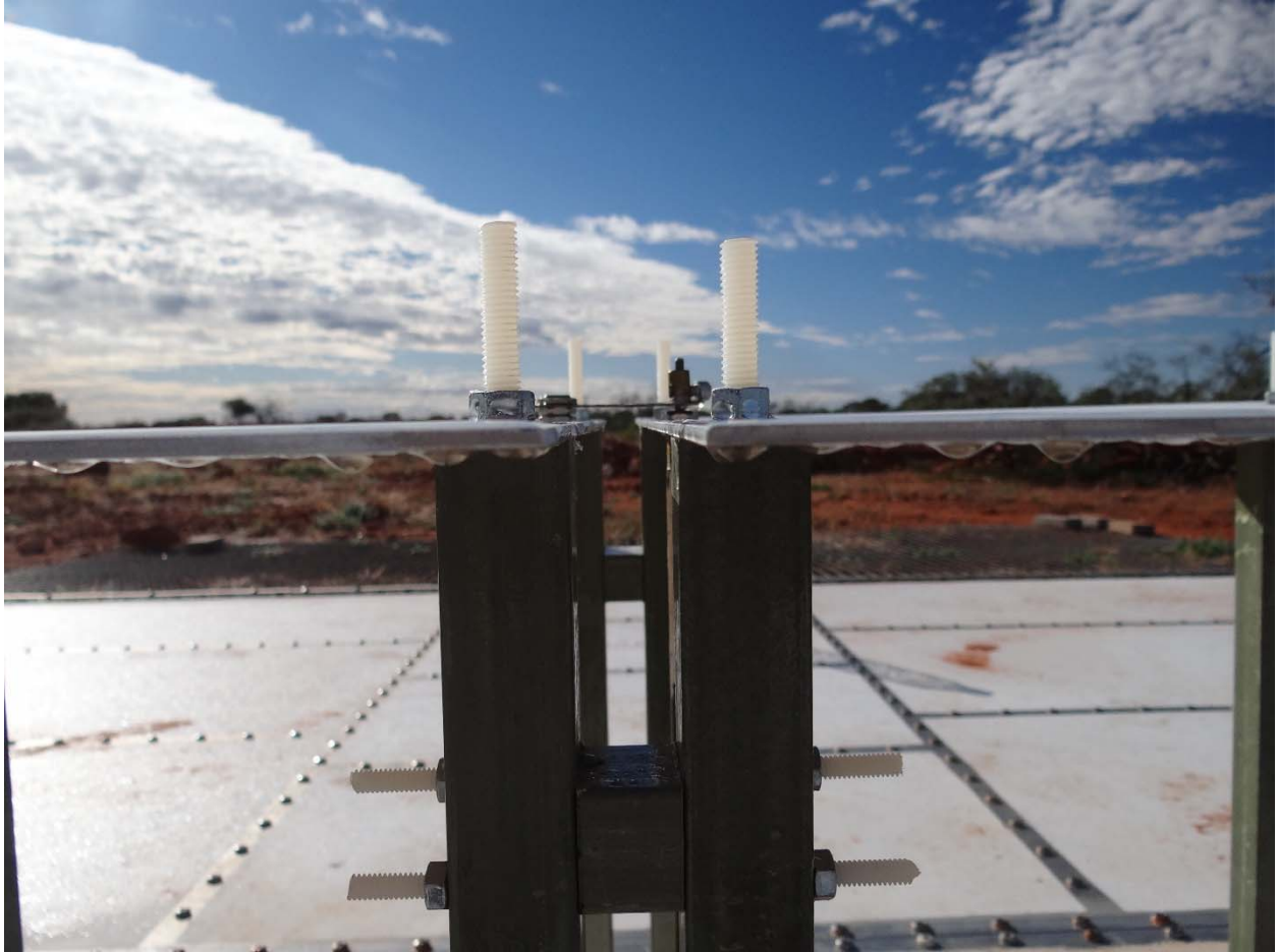
Figure 1. Moisture condensation on blade antenna at the MRO.
