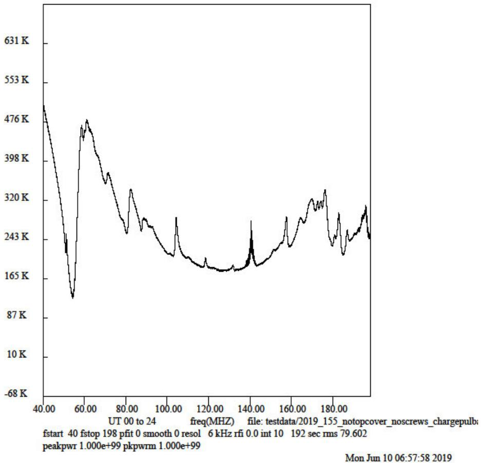
Figure 2. Spectrum with antenna box cover removed.
