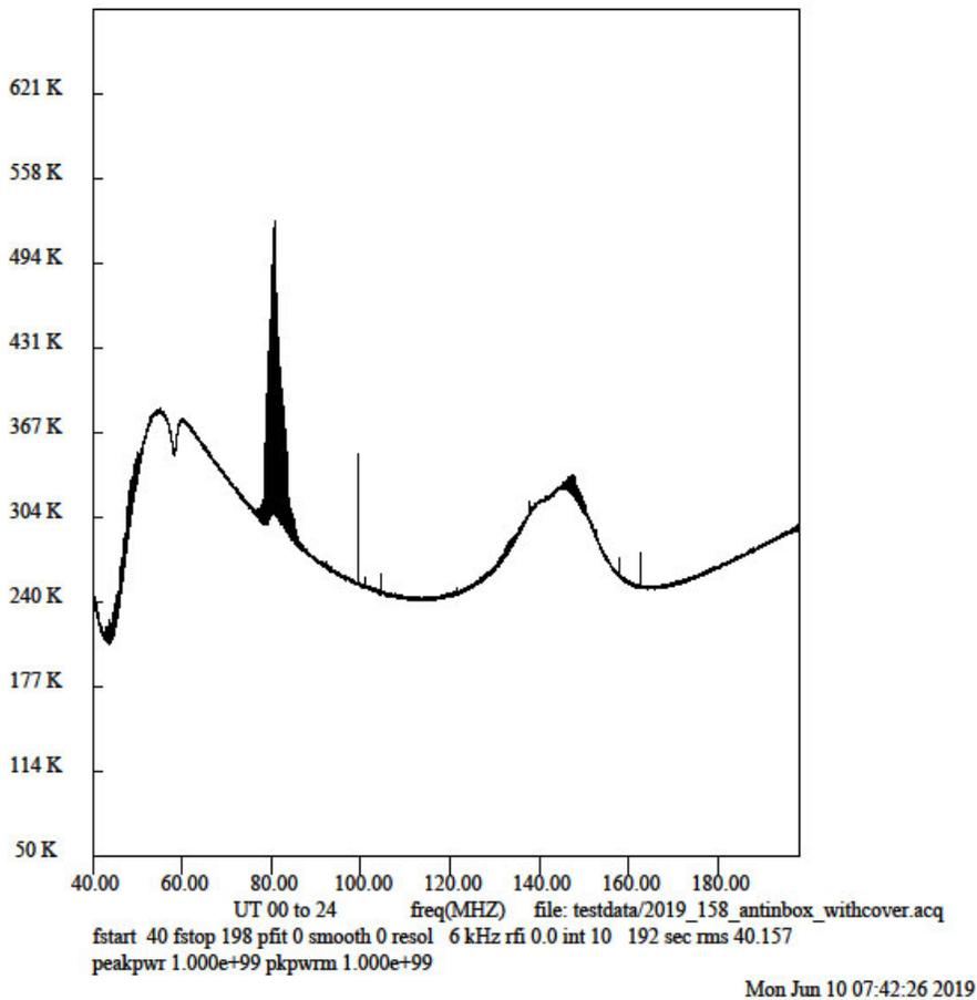
Figure 5. Spectrum with wire antenna in antenna box with box cover in place without screws.
