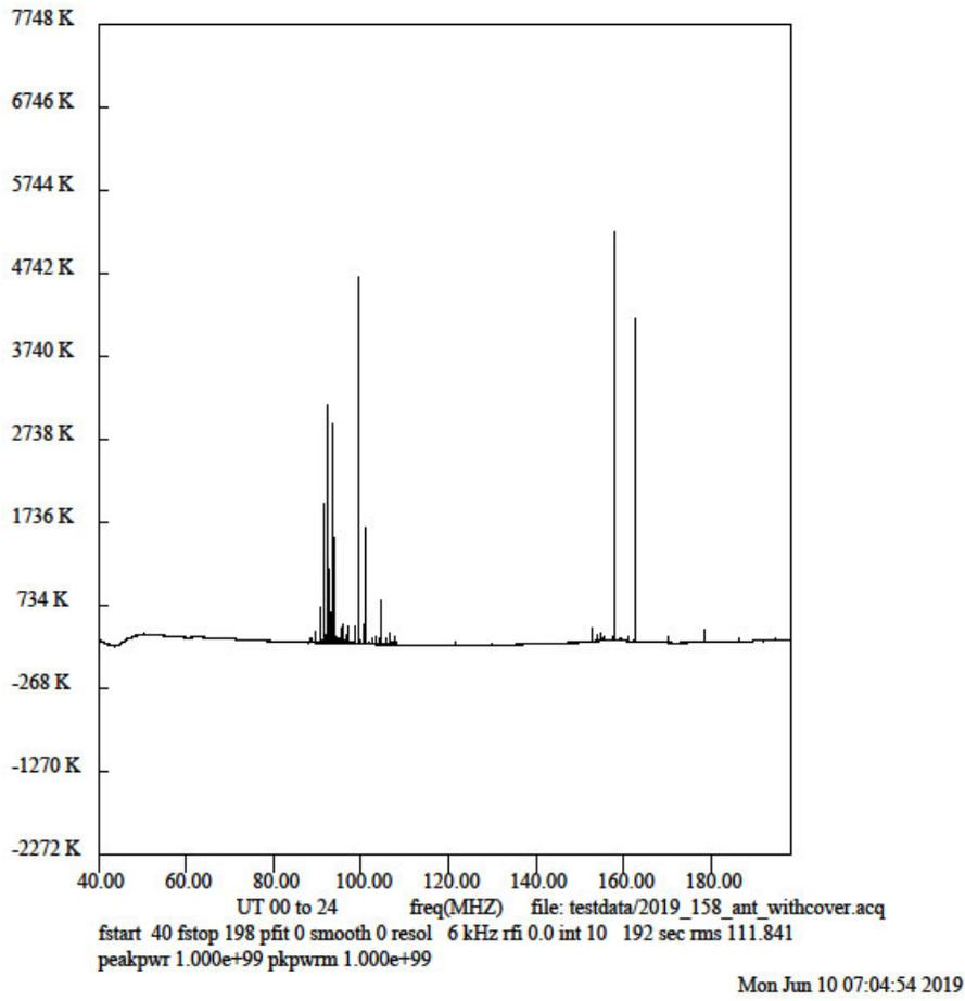
Figure 3. Spectrum in Haystack Observatory screen room.
