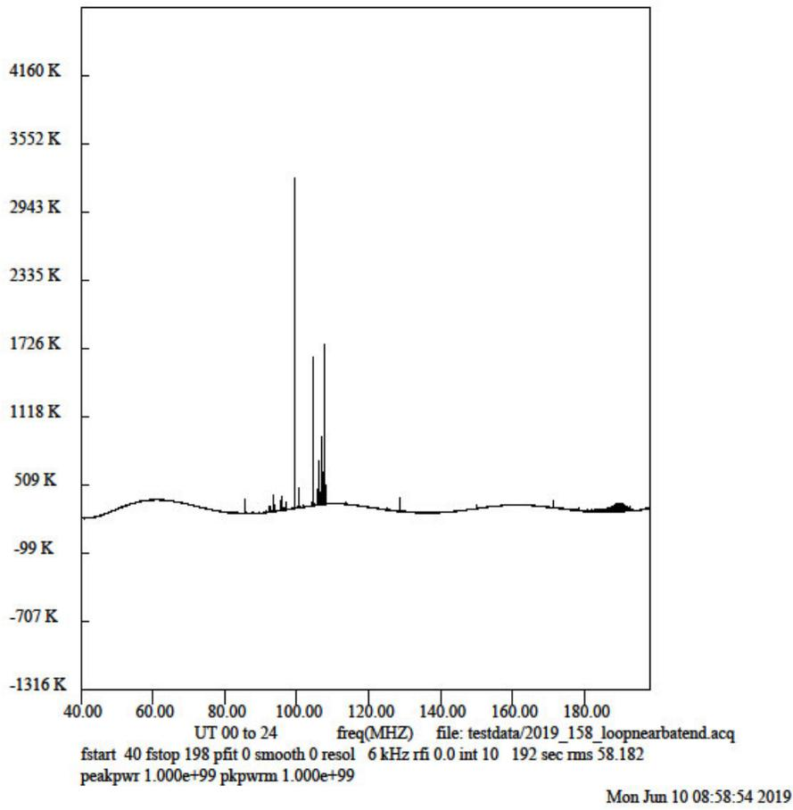
Figure 9. Spectrum using loop antenna after adding ferrites.
