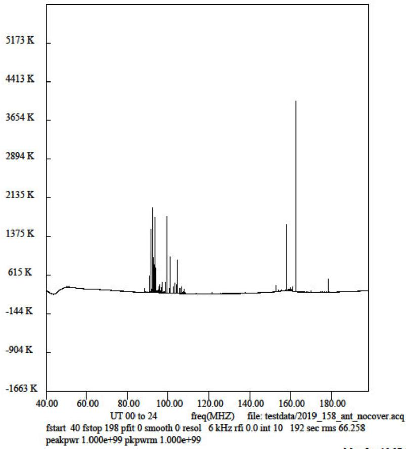
Figure 4. Spectrum with antenna box cover removed.
