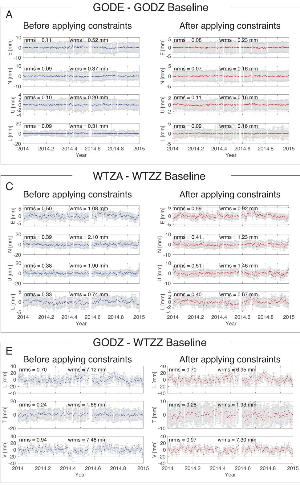
Examples of baseline scatter before and after applying atmospheric constraints for baseline lengths spanning between 0 and 6500 km, in 2014.
