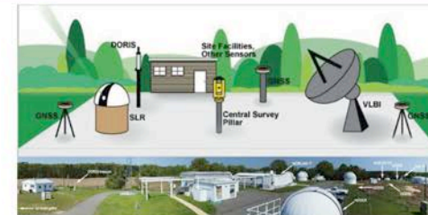
Figure 3: Concept (top) of a GGOS core geodetic site depicting co-location of various instruments from four space geodesy techniques, and a realization (bottom) at the Goddard Geophysical and Astronomical Observatory (GGAO); see Fig. 1). From cddis.gsfc.nasa.gov.
