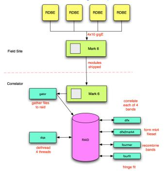
**UC1:** scatter-gather (sg) files are reassembled by gator running on a mk6 and written to NFS-mounted RAID. Files are dethreaded by dqa and written back to RAID. difx correlates each band (= thread) of 16 channels separately, and data are merged by fourmer into single filesets to be fringe fit with fourfit.
