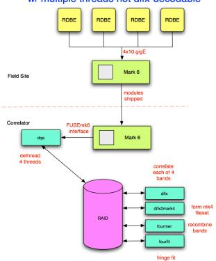
UC2: sg files are reassembled by FUSEmk6 file-system running on a mk6, read into dqa, where the threads are separated into separate files and written to NFS-mounted RAID. difx correlates each band (= thread) of 16 channels separately, and data are merged by fourmer into single filesets to be fringe fit with fourfit.
