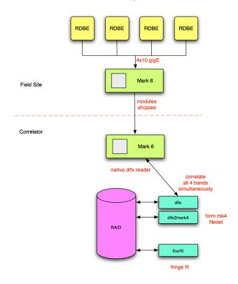
uc4: sg files are reassembled upon reading by difx. This requires code for a native-mode difx datastream handler. It also requires difx to have the capability to correlate multiple (4) vdif threads, each having multiple (16) channels. The data then no longer need to be merged by fourmer, and the output of difx2mark4 consists of single filesets with 64 channels of correlated data. These filesets are then fringe-fitted with fourfit.
