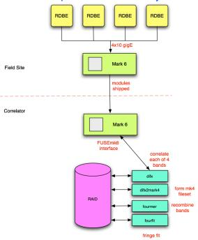
UC3: sg files are reassembled by FUSEmk6 file-system running on a mk6, and read directly by difx. This requires difx to have the capability to correlate multiple (4) vdif threads, each having multiple (16) channels. The data then no longer need to be merged by fourmer, and the output of difx2mark4 consists of single filesets with 64 channels of correlated data. These filesets are then fringe-fitted with fourfit.
