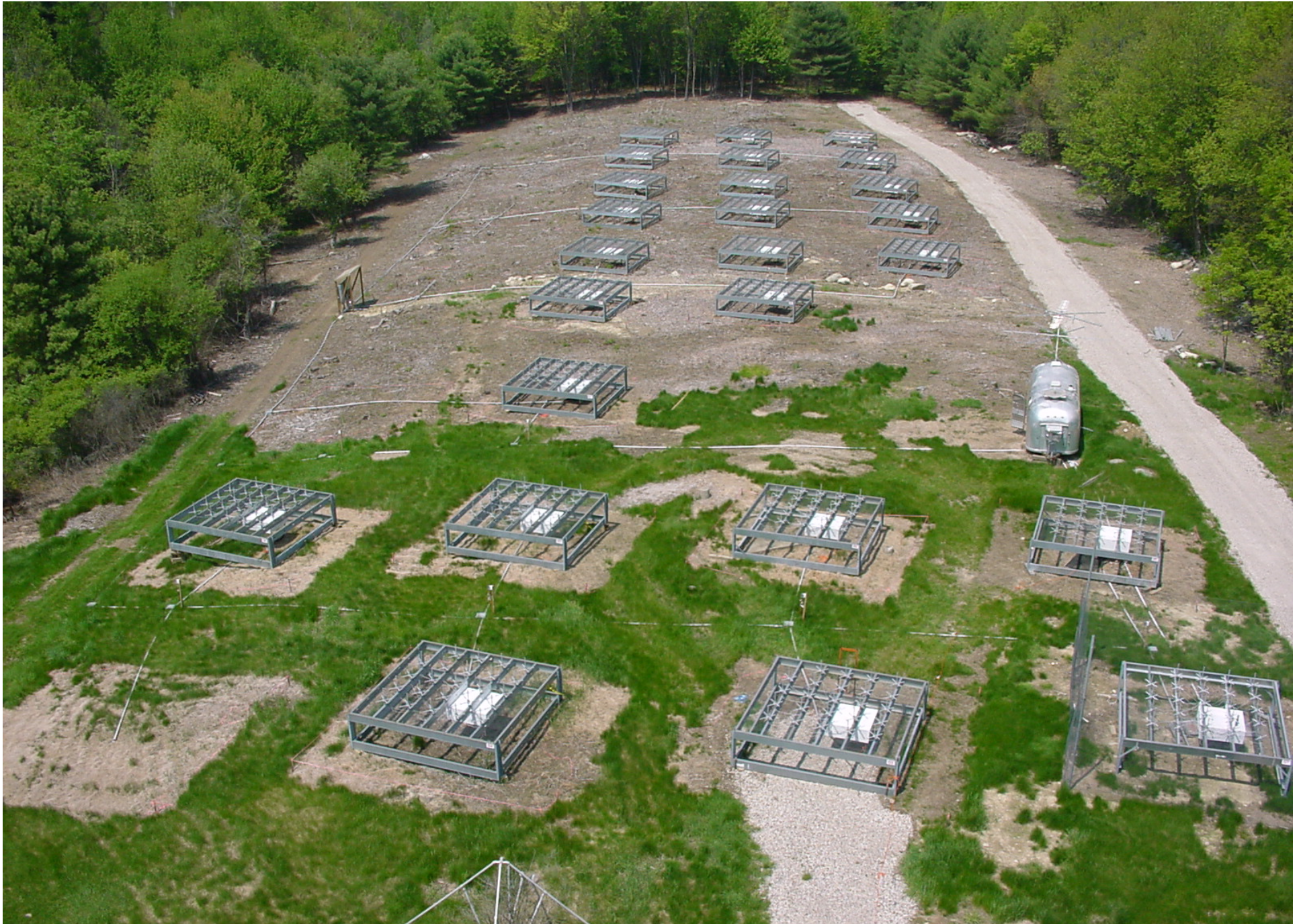
D1 ARRAY of 24 STATIONS EACH WITH 24 CROSSED-DIPOLES
