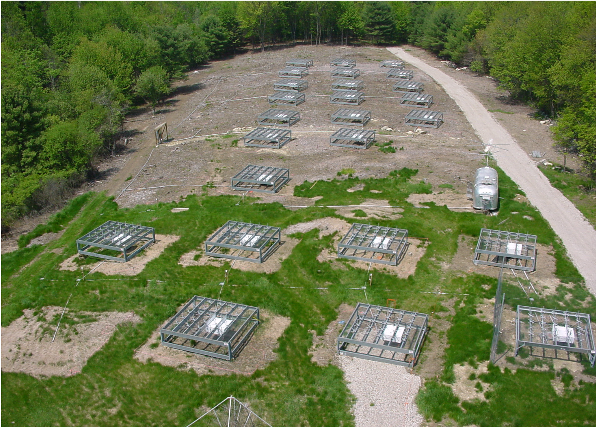
D1 ARRAY of 24 STATIONS EACH WITH 24 CROSSED-DIPOLES
