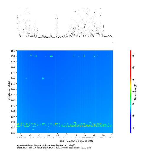
Figure 1. Spectrum from 136 to 151 MHz taken at Mileura. The variable signals from 137 to 138 MHz are from the LEO Orbcomm satellites.
