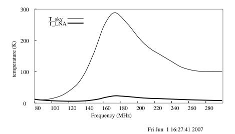
Figure 4. Simulated LNA output for new antenna with new pc board inside an ideal 300 K chamber.
