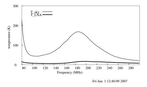
Figure 3. Same as figure 2 but with 270 nH inductor reduced to 100 nH.
