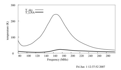
Figure 2. LNA output for new antenna with the new pc board.
