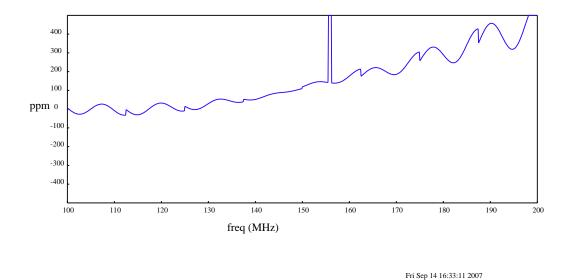
Figure 1. "Stitched" spectrum using 10 MHz bands each calibrated with 3 position switch. The systematics are the result of 100 ppm non-linearity.
