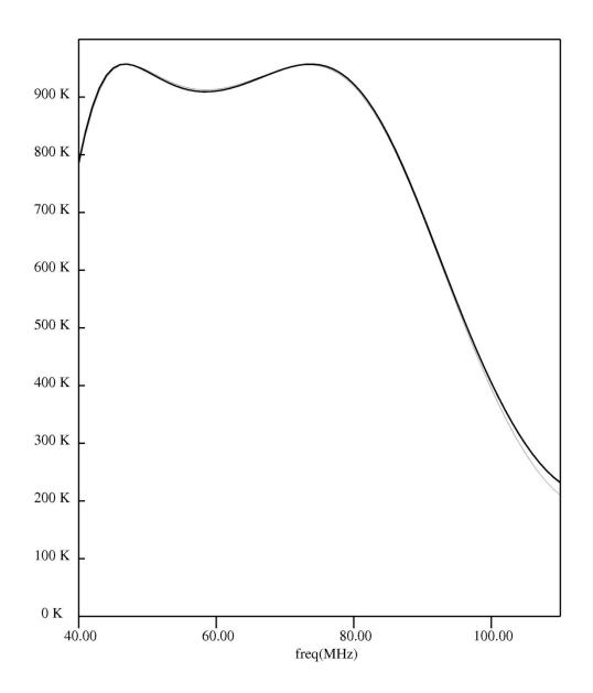
Figure 4. Output temperature of balun connected to antenna in uniform 1000 K sky for 2 models of balan noise. The difference is shown in Figure 5.
