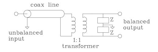
Figure 1. Balun circuit model.
