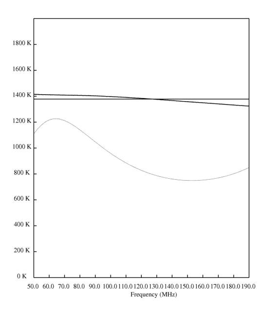
Figure 6. Partially calibrated spectrum prior to correction for the balun. The lower curve is the observed spectrum before calibration. The upper curves are the partially calibrated spectrum and best fit constant of 1377 K.
