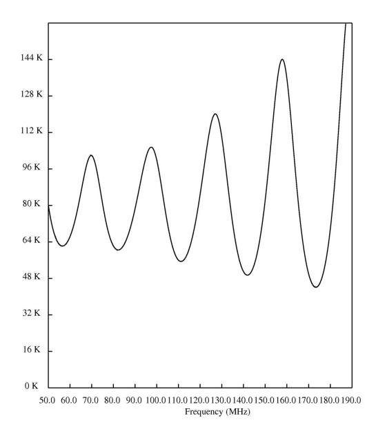
Figure 5. Spectrum of the noise wave calibration cable and fit using 4 term polynomial for each of the 3 noise wave parameters.
