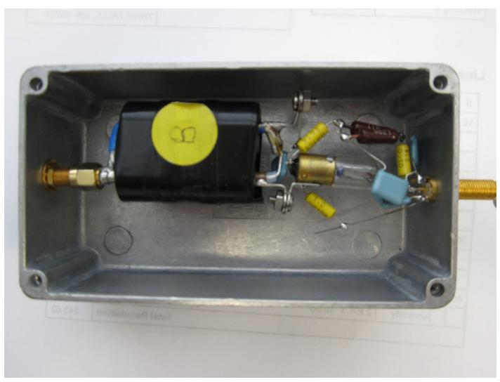
Figure 2. Antenna simulator with balun and hot filament noise source
