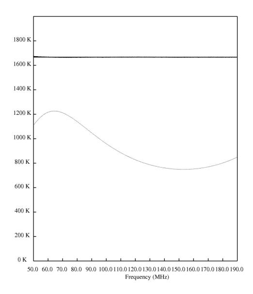
Figure 7. Calibrated spectrum. The average is 1666 K and the rms deviation from a constant is  $1^{\circ}K$ .
