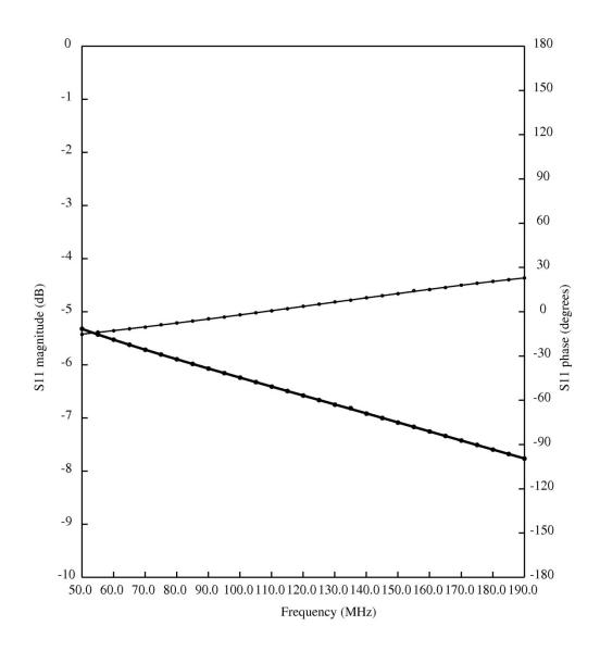
Figure 3. Antenna simulator reflection coefficient. Thick line is the phase. Cures are a polynomial fit to the measurements.
