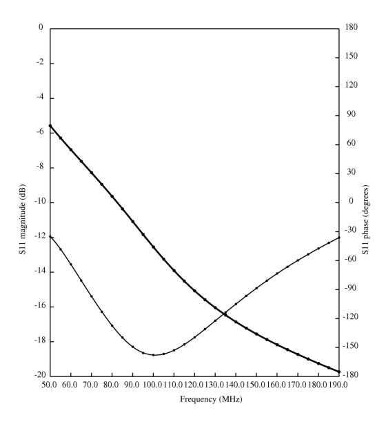
Figure 4. LNA reflection coefficient. Thick line is the phase. Curves polynomial fits to the measurements.
