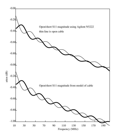
Figure 1. Comparison of VNA cable measurements with results expected from model.
