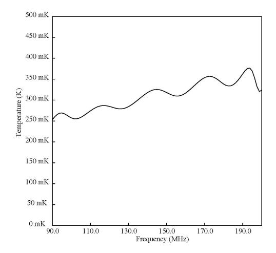
Figure 1. Expected change in spectrum for 10°C increase in temperature.
