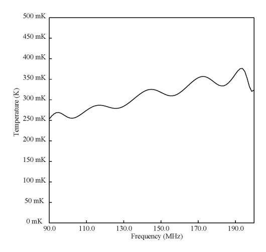
Figure 1. Expected change in spectrum for 10°C increase in temperature.
