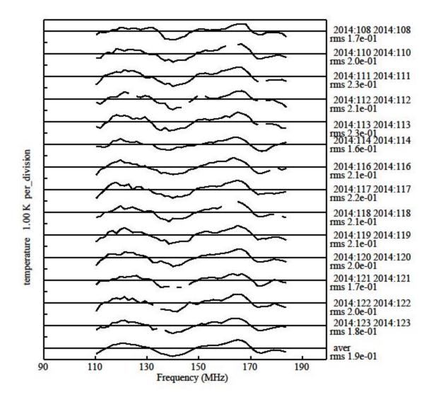
Figure 2. Same as Figure 1 with a wider frequency coverage showing the effect of the frequency dependence introduced by the LNA box.
