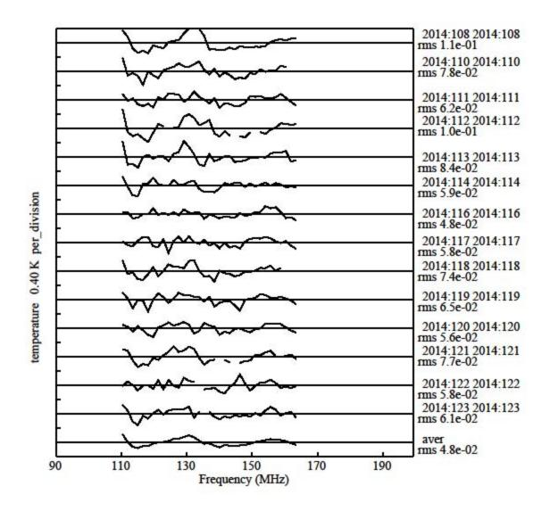
Figure 1. Difference spectra for each day along with average. The values of rms deviation from a constant are given in K. The rms for the average is 48 mK.
