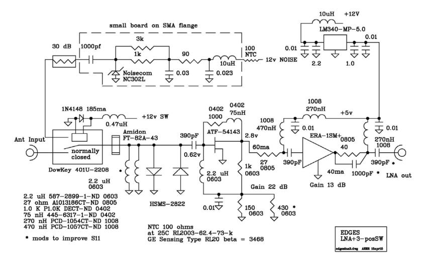
Figure 1. Adjustments to LNA circuit.
