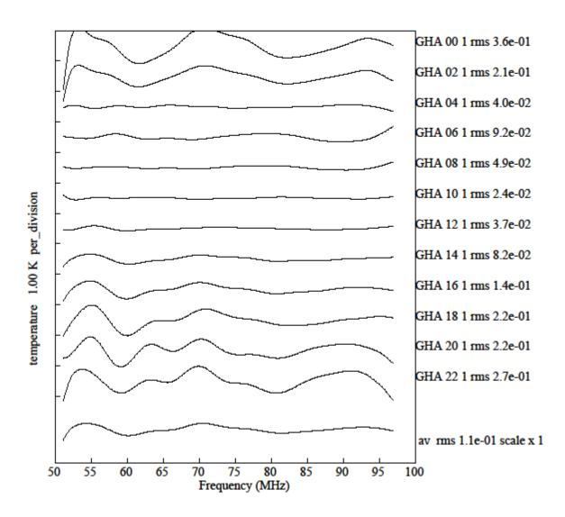
Figure 5. Simulation for  $10 \times 10$  m ground plane on soil with dielectric constant of 13.
