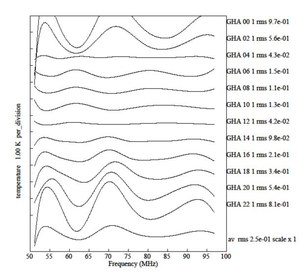
Figure 1. Simulation of beam chromaticity with 5 physical terms removed for 10 m  $\times$  10 m ground plane.
