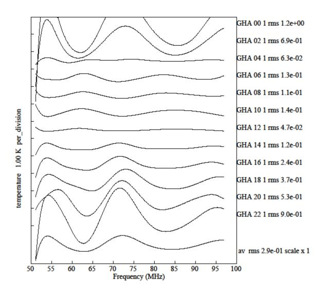
Figure 4. Simulated spectrum for square ground plane of  $9.8 \times 9.8$  m.
