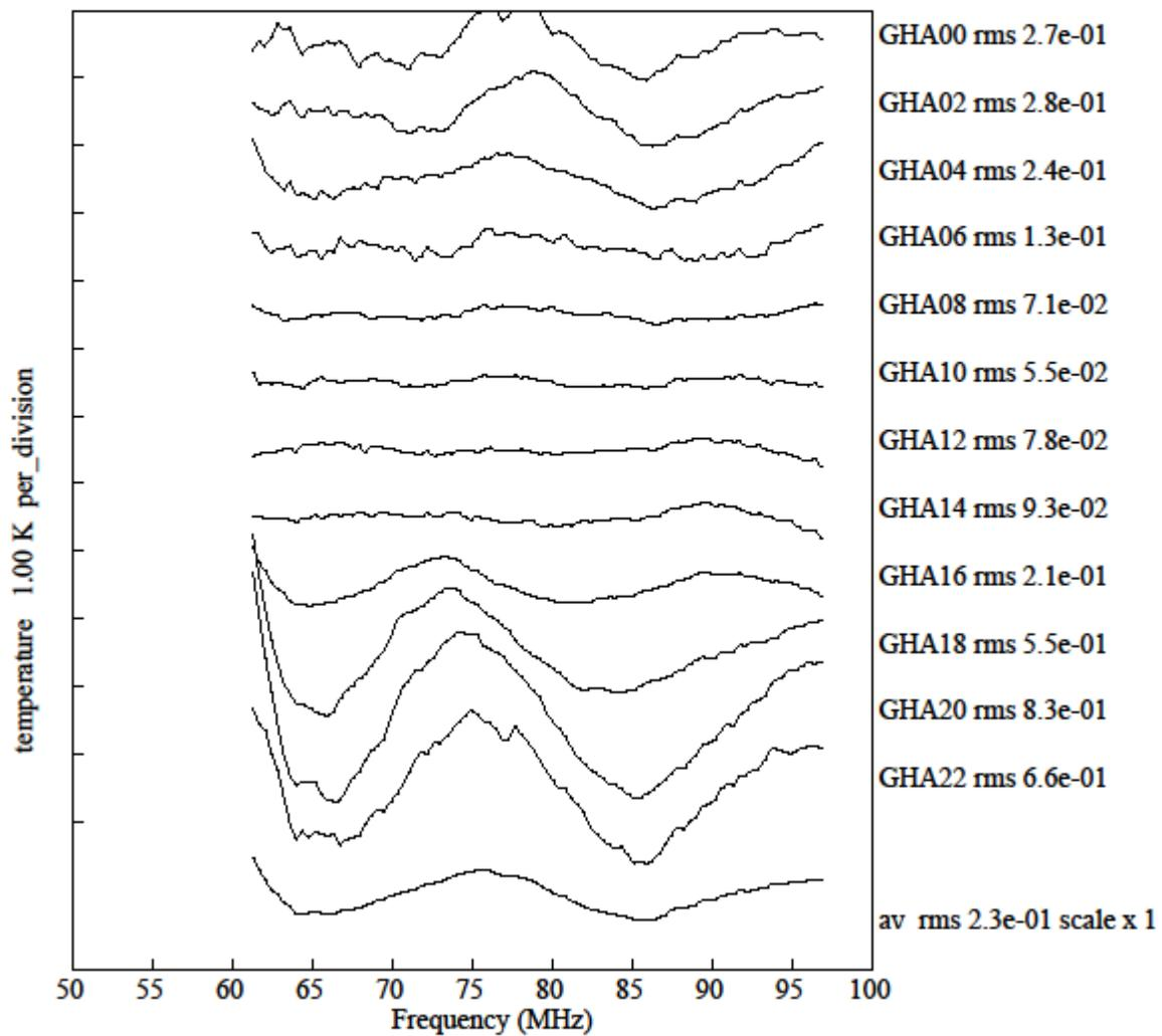
Figure 1. Low band data 4 physical terms removed without beam correction from 2015\_286-2016\_044 averaged over 4 hours at each GHA
