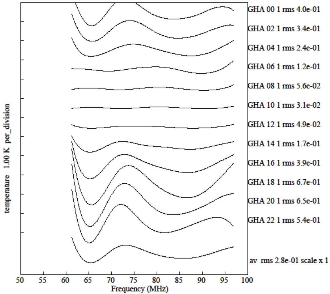
Figure 2. Simulation of beam effects for ground plane  $9.8 \times 9.8$  m. Beam data smoothed with 22 term Fourier series. 4 physical terms removed.
