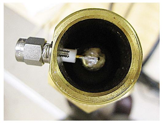
Figure 4. Center conductor soldered to Fairchild microwave SC3792 SMA male connector shown with polystyrene plug removed.
