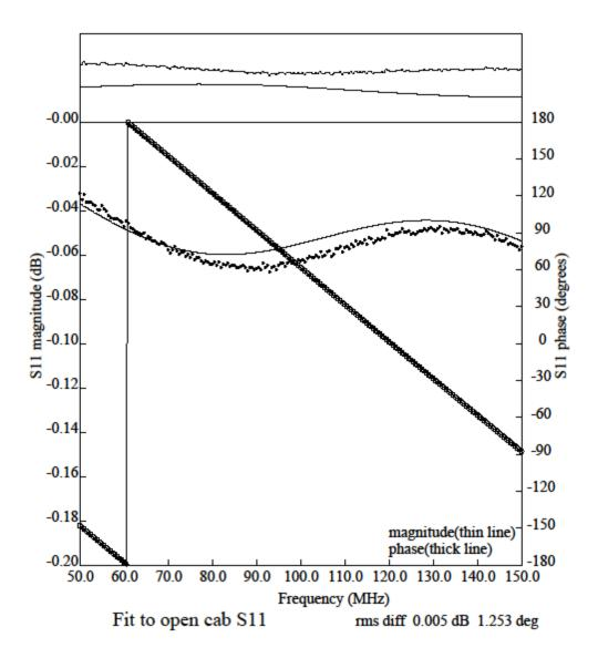
Figure 6. Balun S11 measured with open end.
