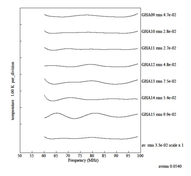
Figure 1. Residual spectra from simulation using 4 term polynomial antenna beams using FEKO of blade antenna oriented NS on extended ground plane with soil dielectric 3.5 and conductivity 2e-2 S/m.
