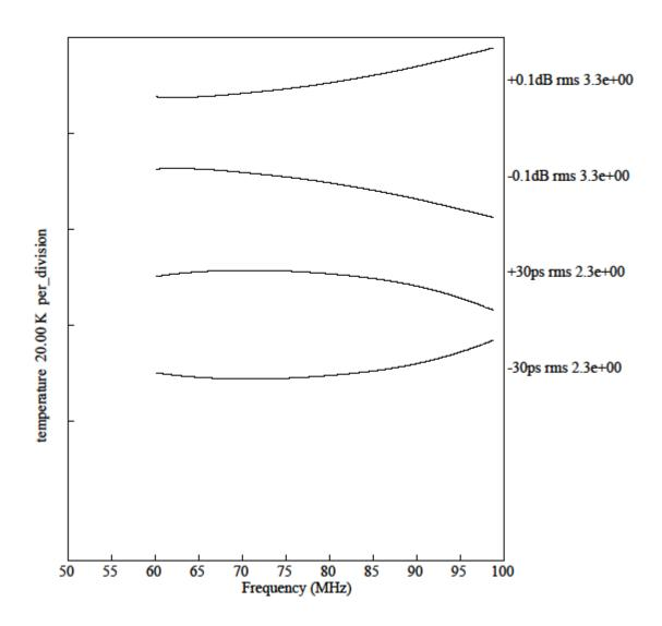
Figure 1. Change in "open" spectrum with a change in LNA S11.
