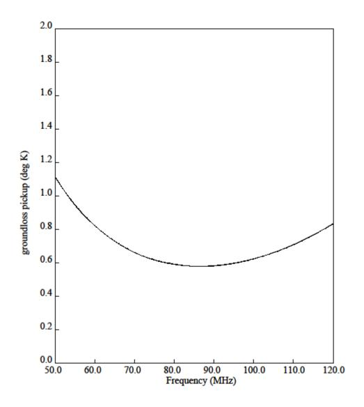
Figure 1. Estimate of the ground loss of the extended lowband ground plane over lossless dielectric of 3.5.
