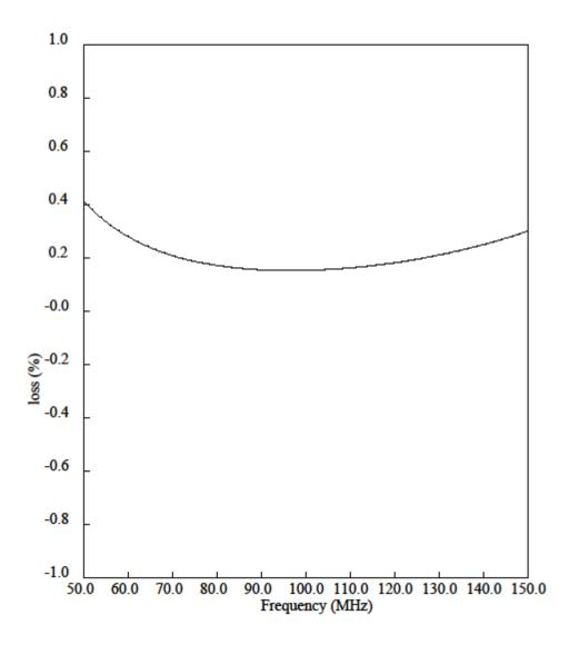
Figure 2. Ground loss in percent for midband antenna on  $30 \times 30$  m ground plane.
