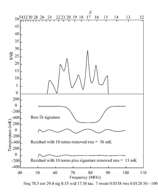
Figure 1. Simulated grid search for signature with 10-terms to remove large errors in antenna S11.
