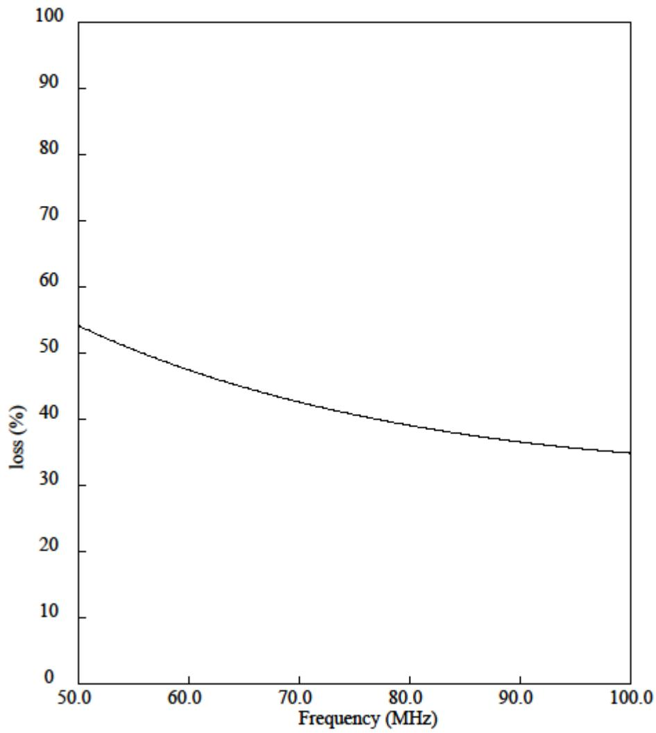
Figure 1. Loss for EDGES-3 at a height of 72 cm above uniform soil with dielectric 3.5 and conductivity  $1e-2$  S/m.
