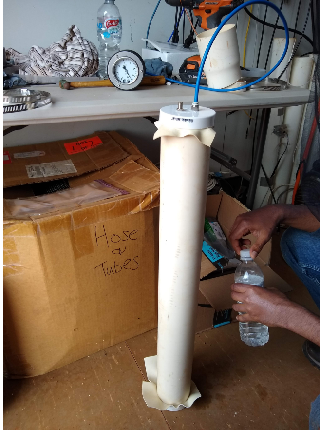
Figure 6: Test chamber used to test end-cap seal before testing the conduit.
