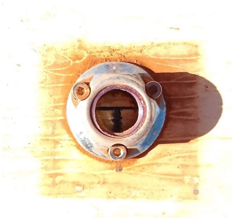
Figure 7: The modified flanged nuts use to attach the threaded nylon rods (withing the fiberglass support legs) to the base-plate.
