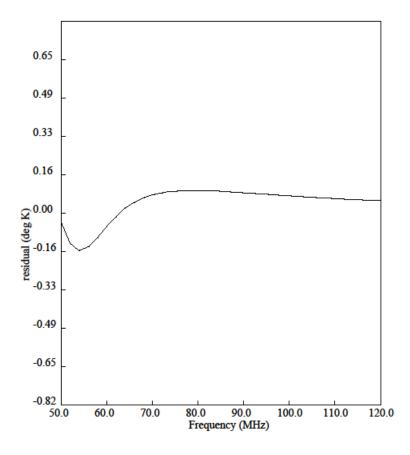
Figure 1. Effect of resistive loss in baseplate with conductivity 1e6 S/m and relative permeability 1.0.
