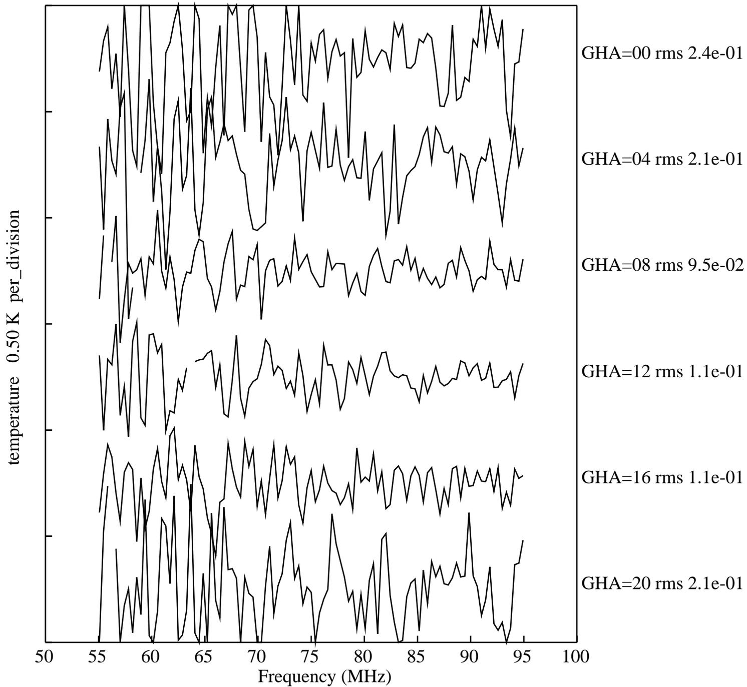
Figure 3. Observed noise in 4 hour blocks of low2-45 data vs GHA.
