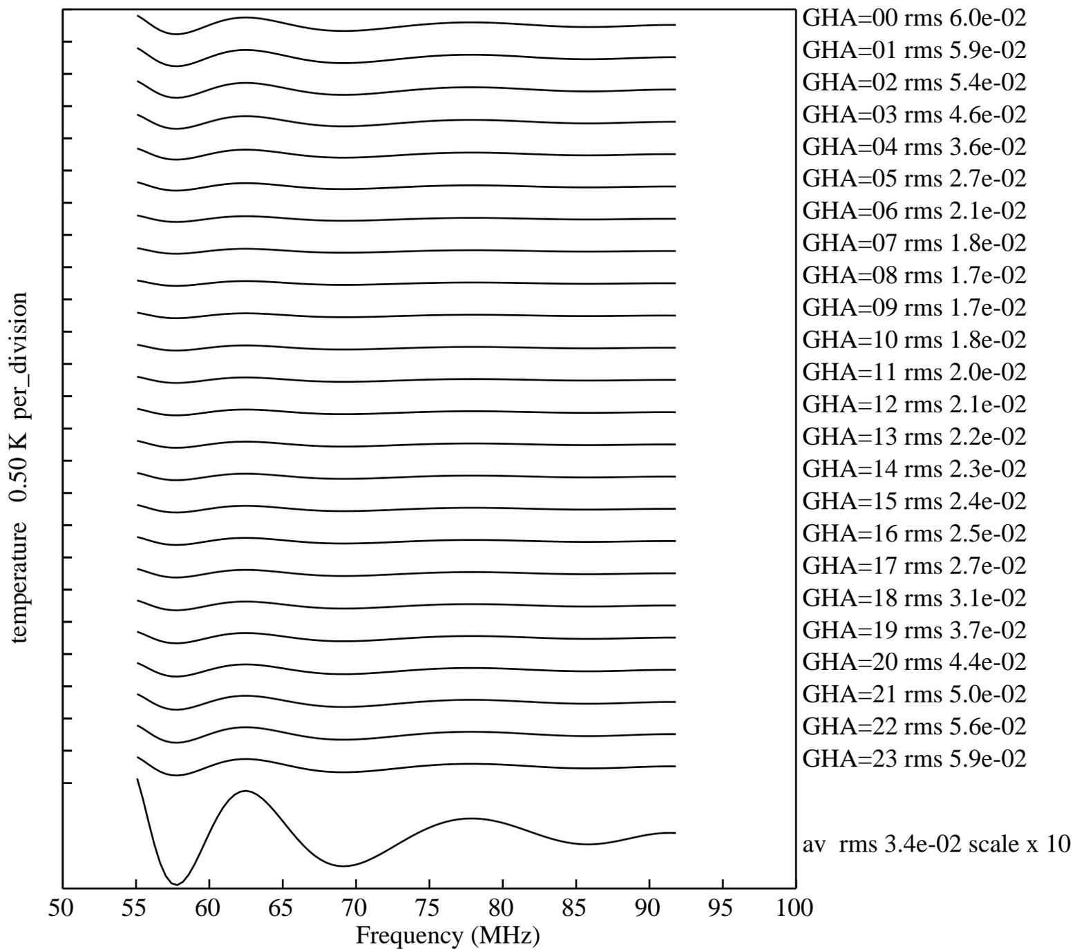
Figure 2. Simulation of the effect of systematic error in S11 or calibration vs GHA.
