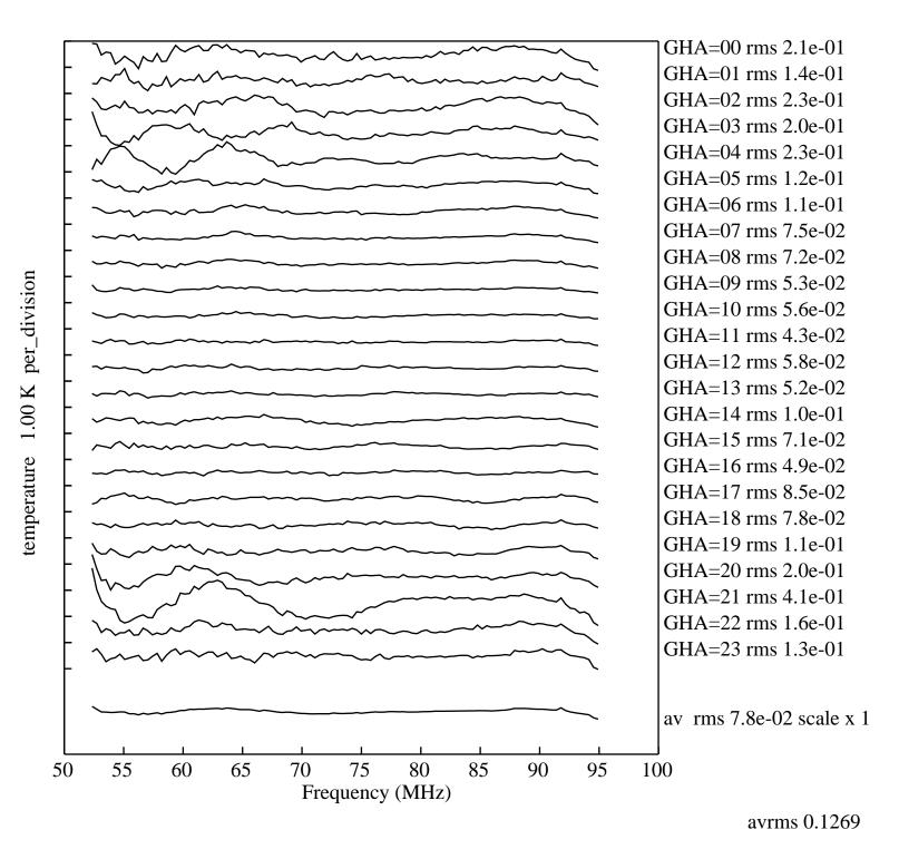
Figure 1. Residuals to low2-45 data from 2020 day 55 to 140 with beam corrections which include the tilt of the ground plane. The foreground and ionosphere are modeled using 5 physical terms.
