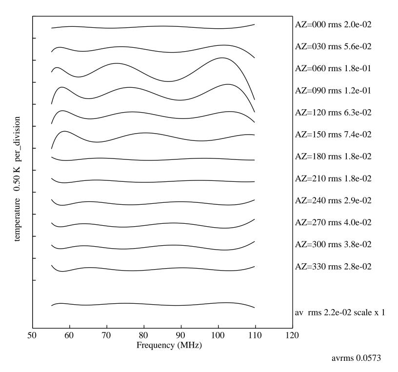
Figure 3. The rms residuals for a simulation of midband beam correction for 5-terms removed for a 6-hour block at GHA=04 hours for a 10 cm bump over 2.5x2.5m in the ground plane with center 5m from the antenna at different azimuths.
