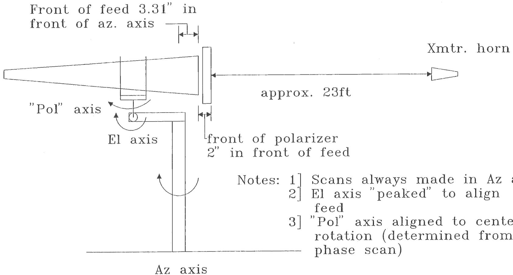
Figure 1. Antenna range set-up
