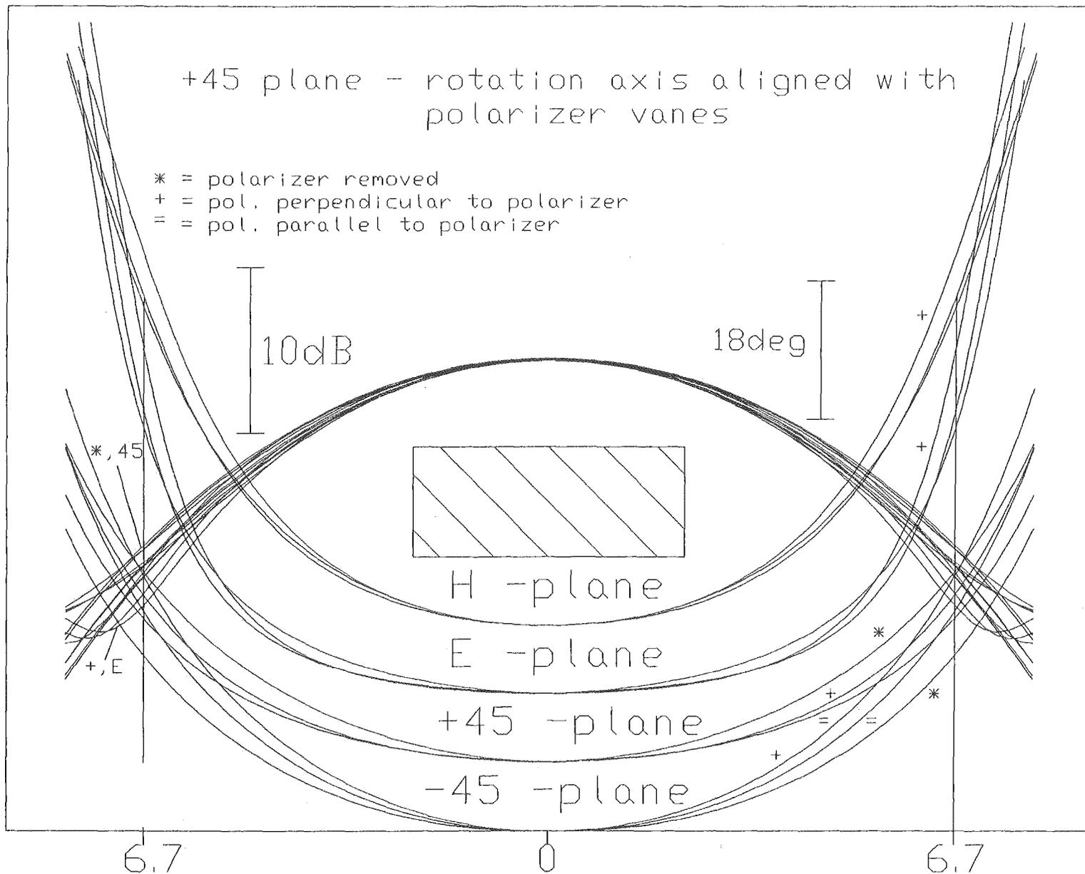
Figure 2. Holography feed phase and amplitude
