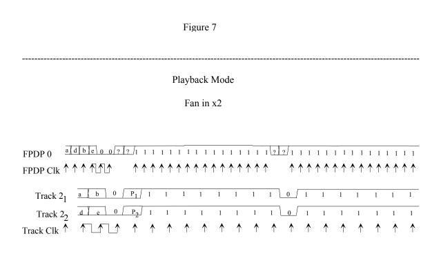
NOTE: FPDP rate is set on output board. Track clock and FPDP clock are derived from a programmable oscillator on the output board.
