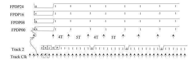
NOTES: FPDP Clock is derived from Track Clock, which is generated by Output Board. Pipeline delay from FPDP0 to Track 2 is shown as two periods of Track Clock.
