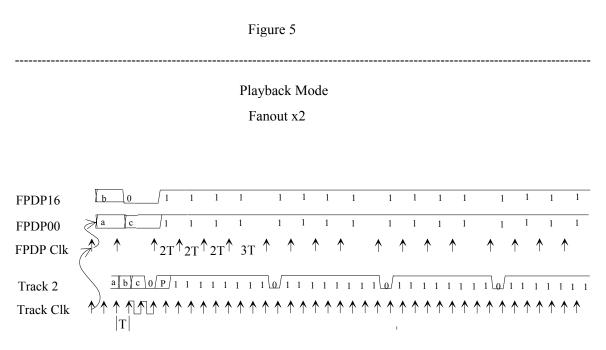
NOTES: Pipeline delay of T from FPDP00 to Track 2.
