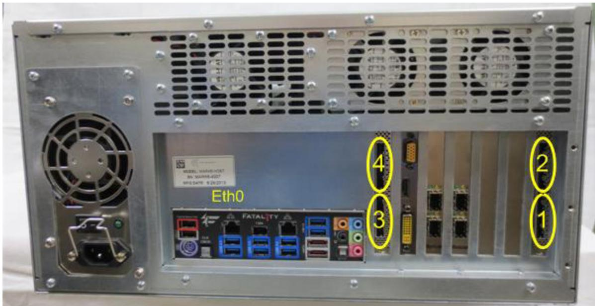
Figure 1 Mark6 Host Bus Adapter to Slot Assignments
