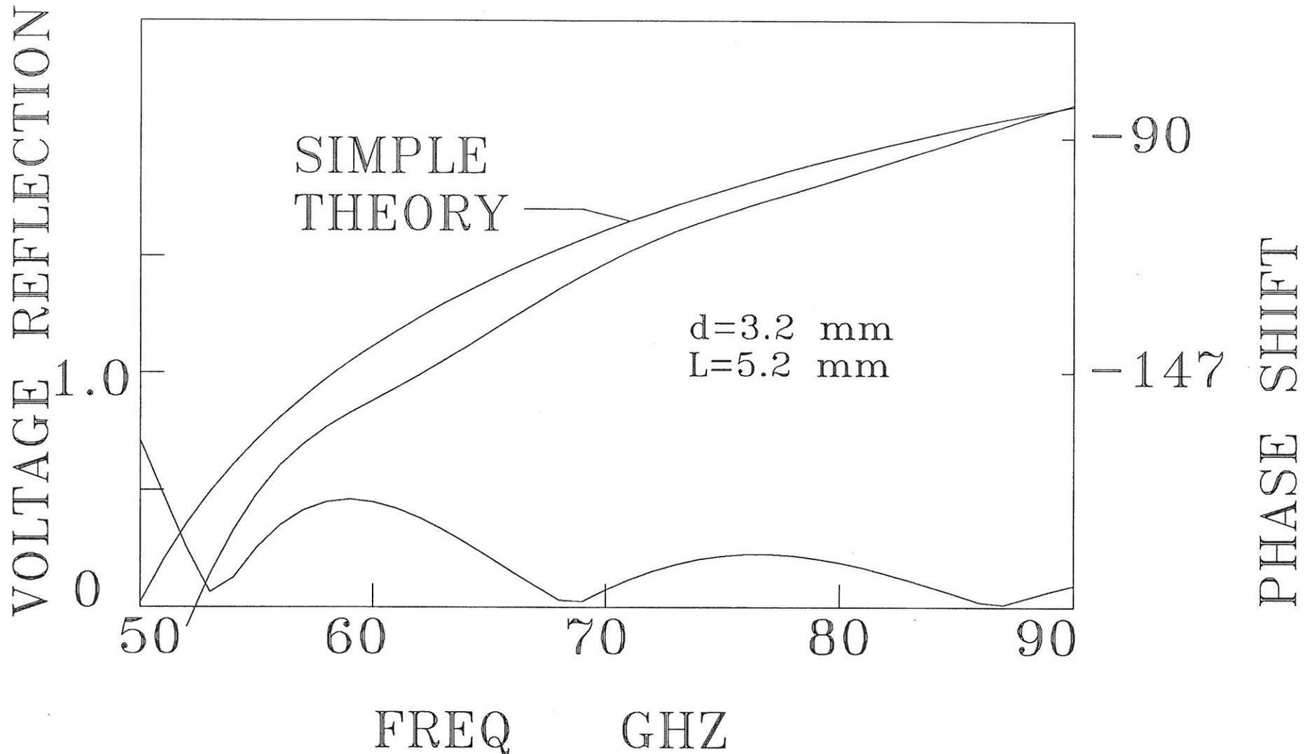
FIGURE 3 POLARIZER PHASE SHIFT AND LOSS USING NUMERICAL SOLN.
