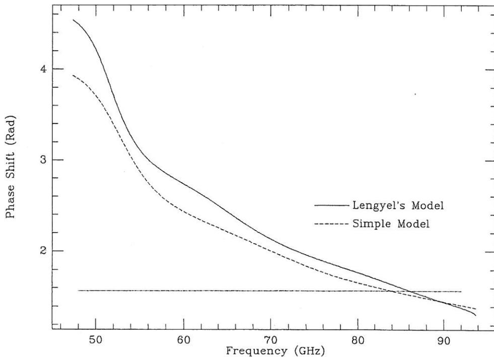
Figure 5: Comparison of Lengyel's reflection and phase shift with those of the simple treatment.
