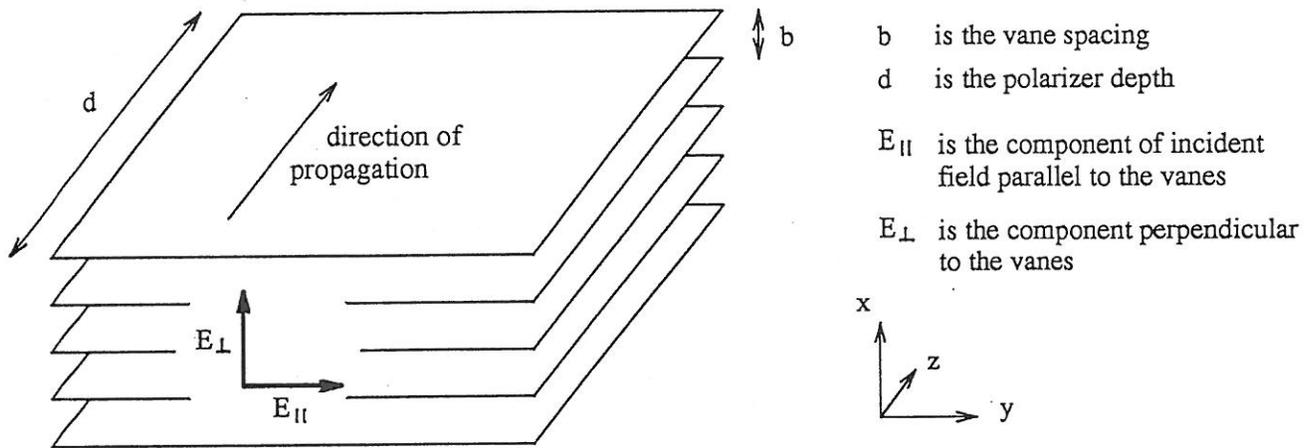
Figure 1: Schematic view of polarizer
