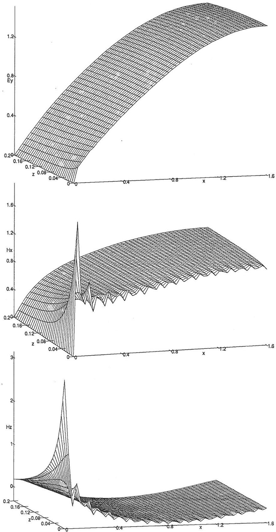
Figure 3:  $E_y$ ,  $H_x$ ,  $H_z$  Fields just inside the metal vanes.  $x$  ranges from vane surface to midway between vanes. Spatial dimensions in mm.
