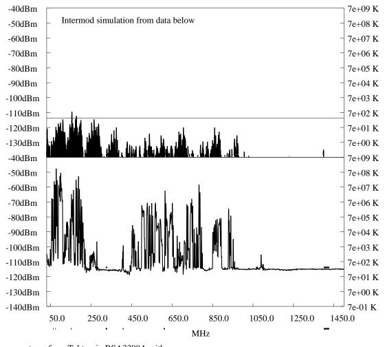
spectrum from Tektronix RSA3308A with preamp start 2005:079:00:01:19 stop 2005:079:12:11:45 resolution 1000.0 kHz
