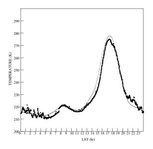
The thin light trace is the predicted temperature obtained from the sky model. The figure shows that despite the lack of load switching the gain is stable enough that continuum RFI is quite apparent at the 5 to 10K level or an equivalent RFI temperature (for an isotropic antenna) of under 1K.
