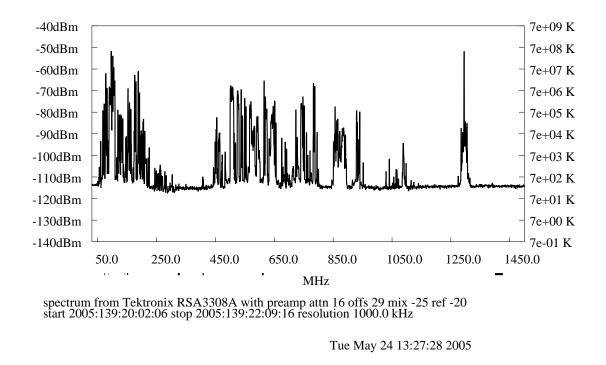
Figure 3. Spectrum with added attenuation before the mixer to improve the dynamic range.
