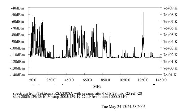
Figure 1. Spectrum with intermodulation products
