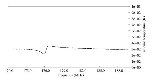
spectrum from Acqiris with preamp attn 0 fpgatm 39.3 degC start 2006:183:18:13:22 stop 2006:183:18:18:52 resolution 122.0 kHz
