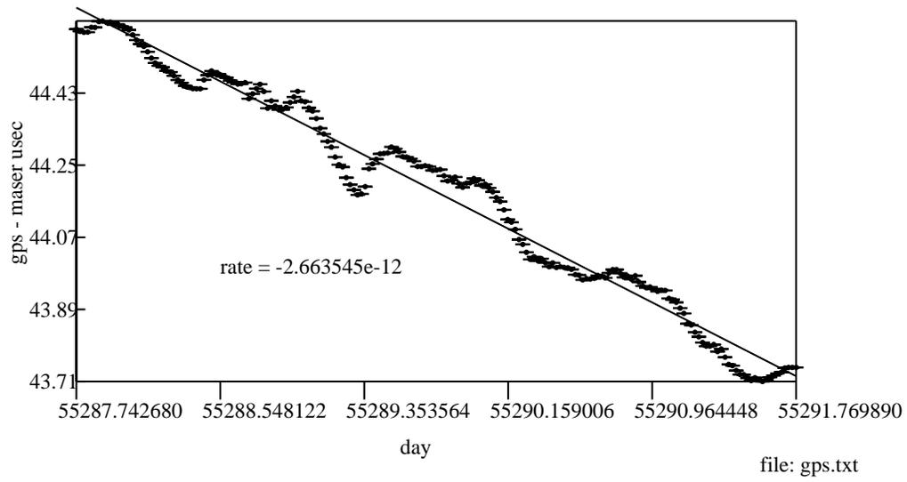
Figure 5. Shows the rate of the maser relative to GPS.
