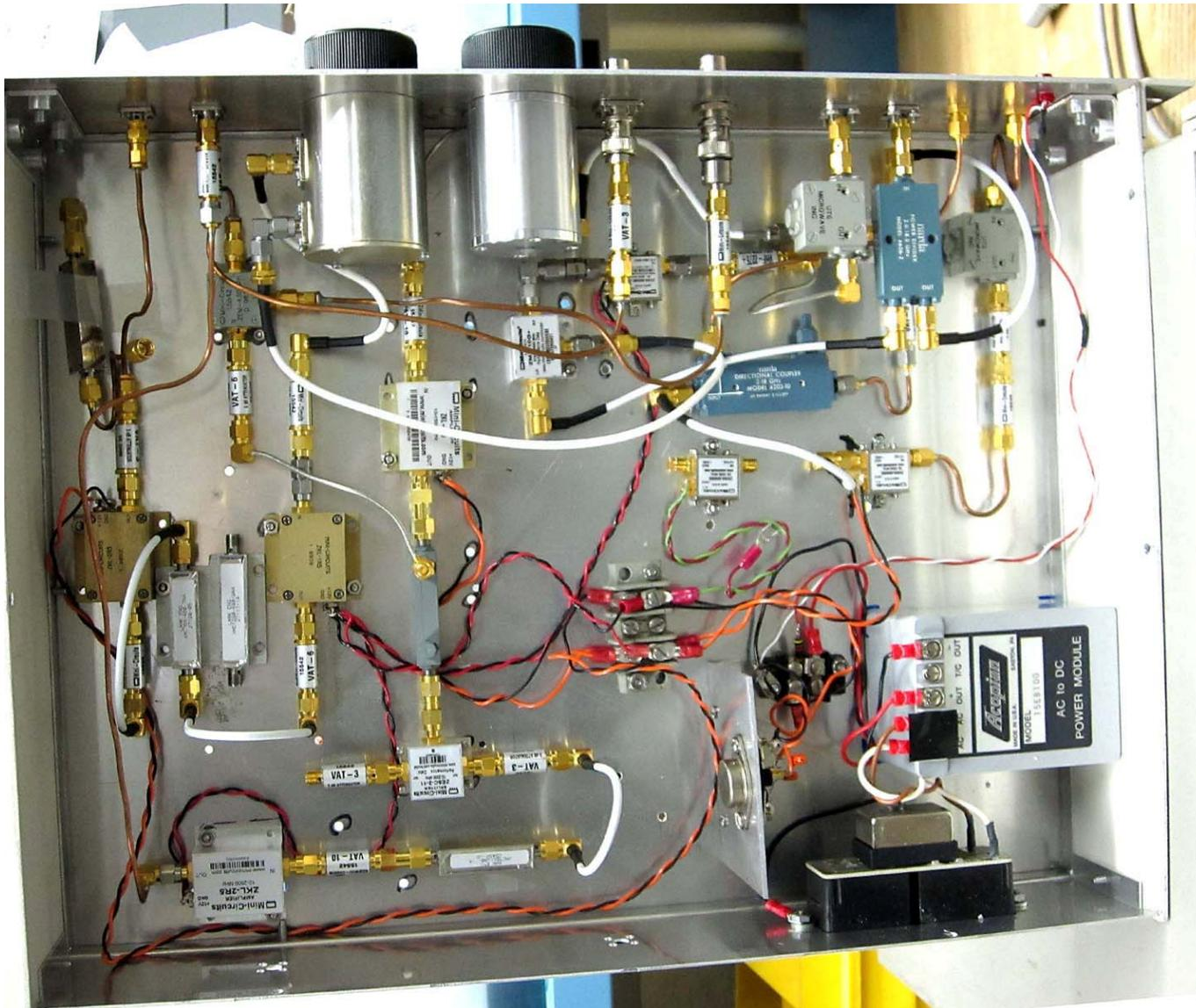
Figure 3. Down converter modified for dual channel
