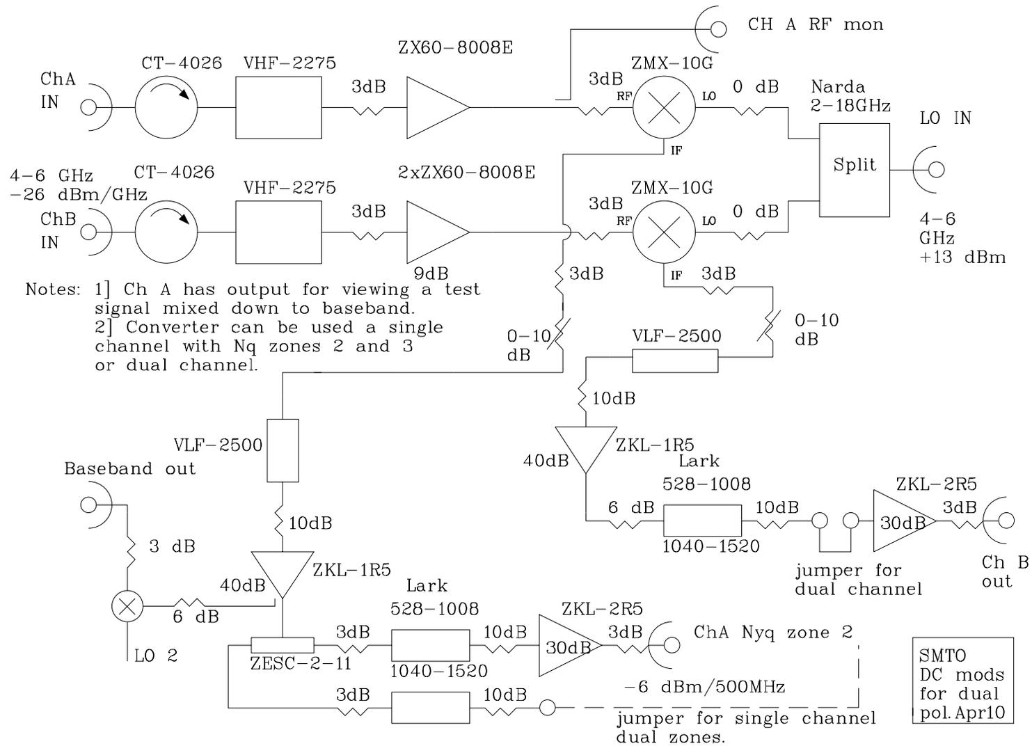
Figure 2. Block diagram on modified downconverter
