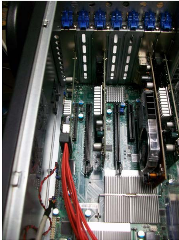
Figure 7.4: The data packets arrive on the 10 GbE PCI-Express card at the center of the picture, and are ultimately stored to disk via the I/O card on the left. The video card and spare 10 GbE card at the right are unused.
