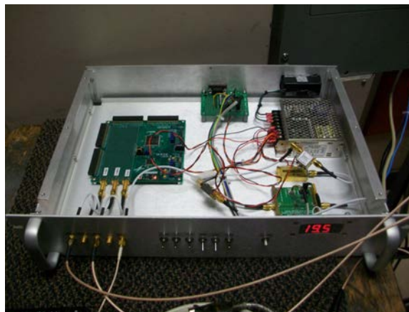
Figure 7.1: The noise source used in these tests provides suitably amplified noise, 5 MHz and 1 PPS signals on 3 cables.
