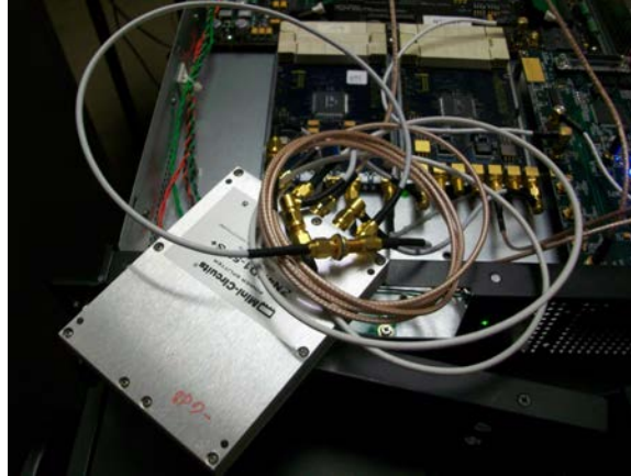
Figure 7.10: Three cables of various lengths were inserted on three of the four splitter outputs to produce different single-band delays on the various baselines.
