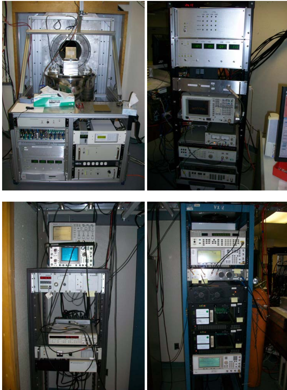
Figure 2: The 230 GHz receiver, support rack, and two VLBI racks are unchanged since previous years except for the insertion of one RDBE-H, two Mark5C recorders, and a digital oscilloscope for DOT monitoring.
