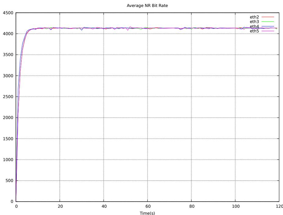
Figure 5: A plot of the instantaneous network packet processing rate for a 2-minute recording.
