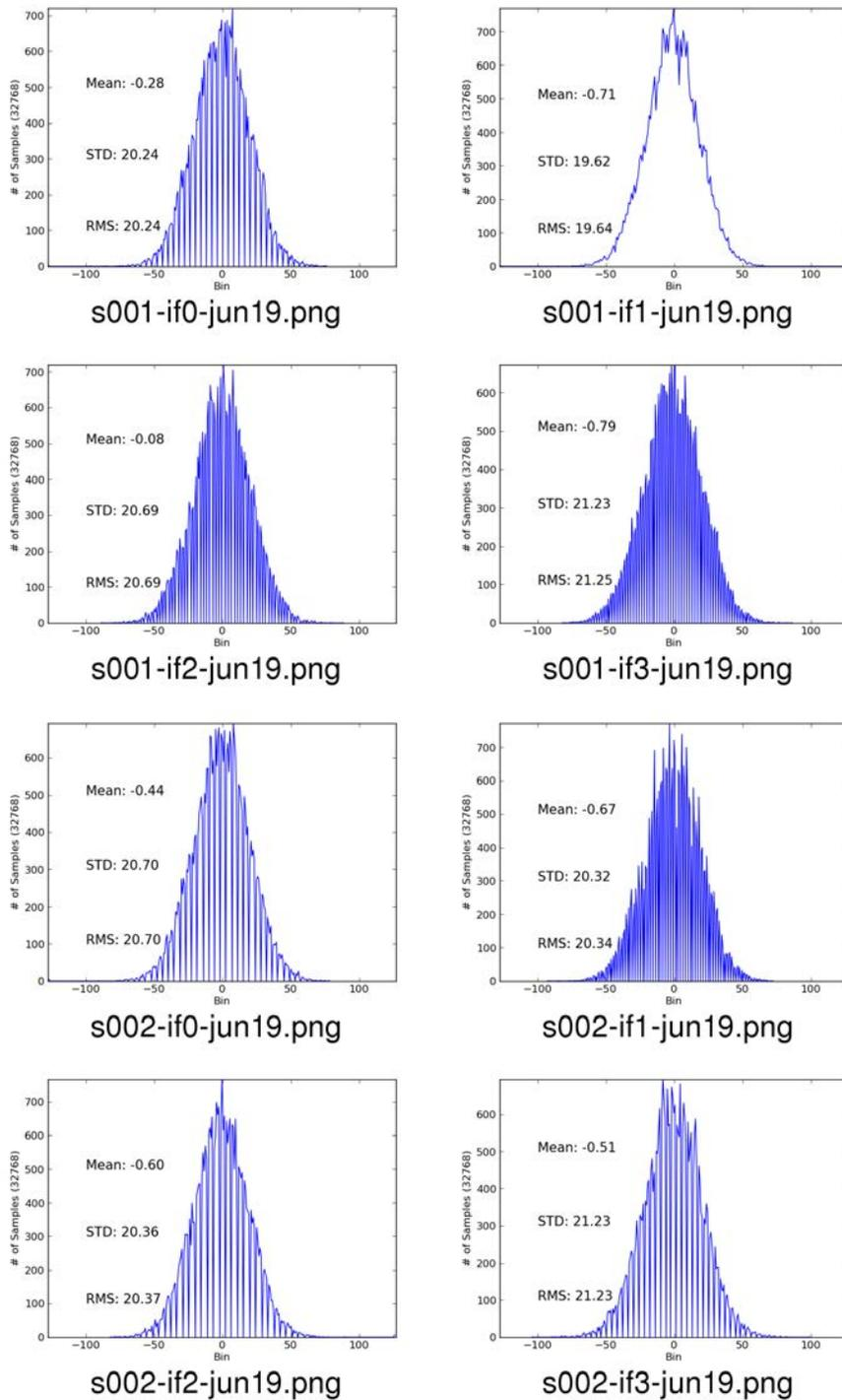
Figure 2: Raw ADC data from the two RDBE-S units (RDBE-S001 and RDBE-S002) at Westford for its 4 IFs.
