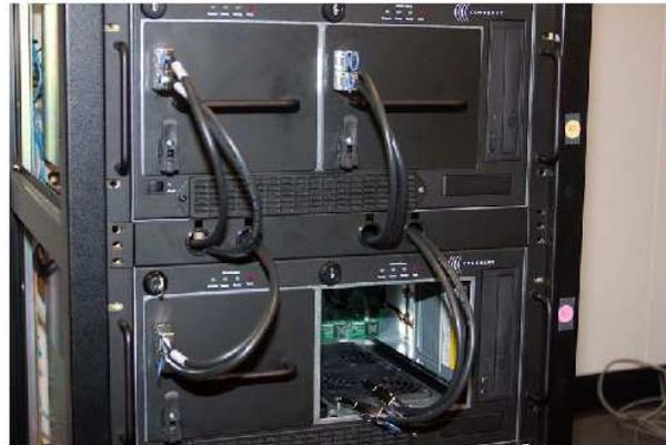
Figure 4: The Mark6 prototype hardware used at Westford. The host computer and 2 disk packs are in the upper 4U module; the 2 additional disk packs are supported by the lower 4U module. A 1U separator provides a cable paths to the host RAID cards.
