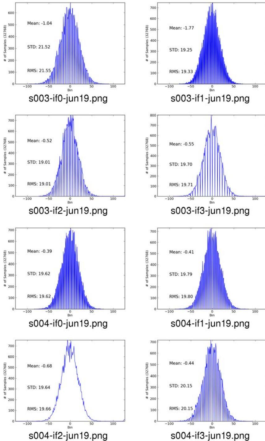
Figure 3: Raw ADC data from the two RDBE-S units (RDBE-S003 and RDBE-S004) at GGAO for its 4 IFs.
