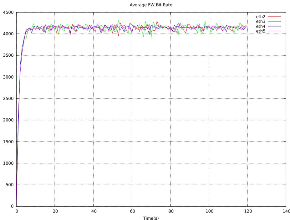
Figure 6: A plot of the instantaneous file write rate for a 2-minute recording.
