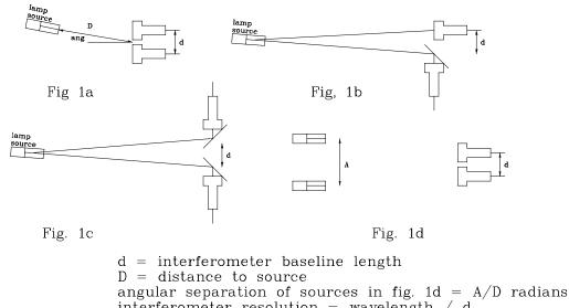
interferometer resolution = wavelength / d wavelength = 2.5 cm (frequency = 12 GHz)
