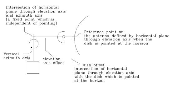
Elevation and dish offsets needed to account for changes in interferometer baseline with antenna pointing
