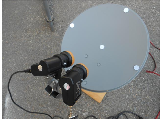
the atmosphere. The system was calibrated to observe the 13.4 GHz OH line using an LNBF with a 12 GHz local oscillator.
