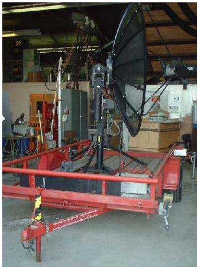
Figure 5-1: An example of a trailer mounted telescope. (Image from MIT Haystack [www.haystack.edu](http://www.haystack.edu))
