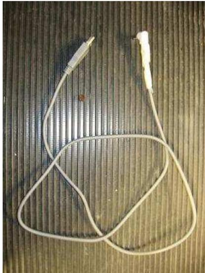
Figure 3-6: The new mutant cable! With a USB terminal and a standard power connector terminal.
